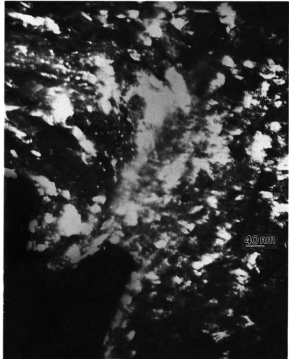
Figure 3. Macro-spiral close to the interface with YSZ substrate formed in the film deposited at T_s = 740^\circ\text{C} (dark-field image). Each "wind" corresponds to a separate screw dislocation.
